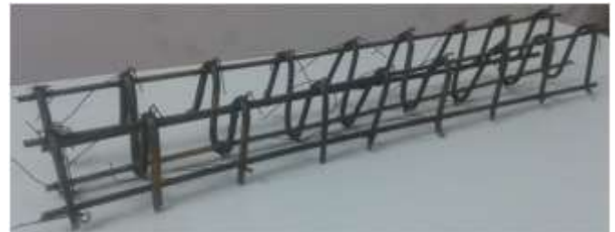
"V" Shaped Reinforcement Profile
