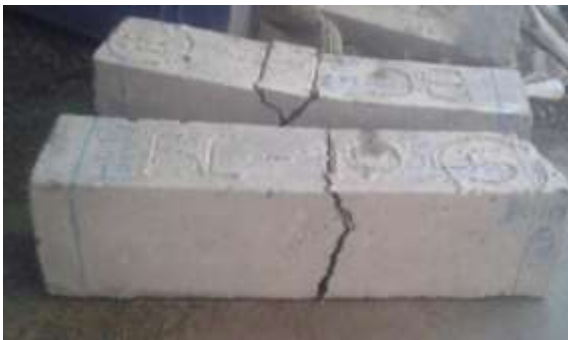
Failure pattern of reinforced concrete beams
